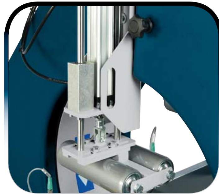
INFEED AND OUTFEED PNEUMATICALLY OPERATING TOP PRESSURE UNITS The vertical pressure units automatically settle in order to ensure a correct stabilisation of the product. The cylinder stroke can be adjusted manually to adjust the pressure on the products of different heights.
