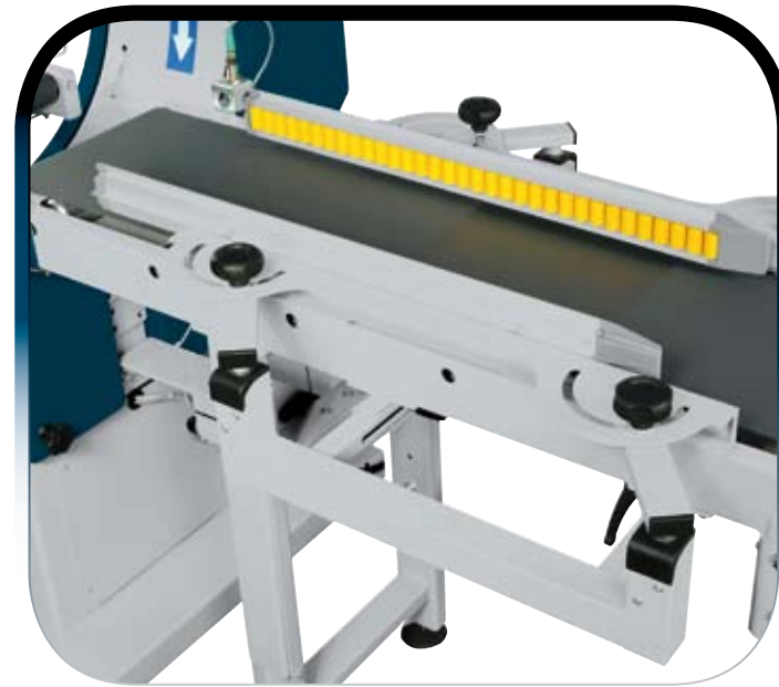
INFEED AND OUTFEED SIDE GUIDES Infeed and outfeed side guides can be manually adjusted to better centre the products of different widths. This operation can be easily done using the available knobs. The product runs smoothly during the wrapping cycle thanks to the presence of idle rollers.
