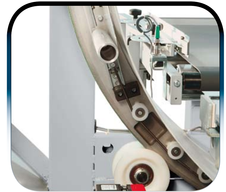
FILM TENSIONING UNIT The tensioning unit present in the 1200 version, guarantees optimal use of the film during the wrapping process. This feature is obtained using a mechanical dancer unit.
