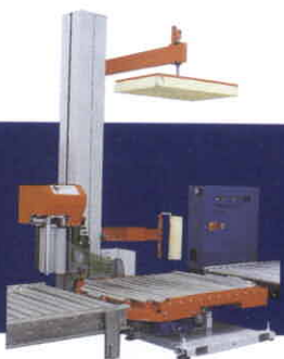
Fully automatic turntable machine
